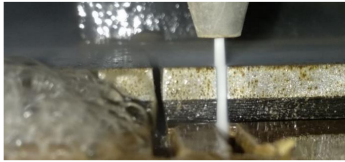
Figure 1. Abrasive water jet machining of a hybrid structure Steel/carbon fiber-reinforced thermoplastics (CFRTP).
