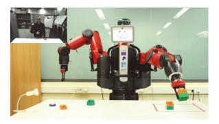
Fig. 11. At the end of the verification task the operator (inset image shows the view from the robot front-facing camera) makes a gesture of approval to the robot.
