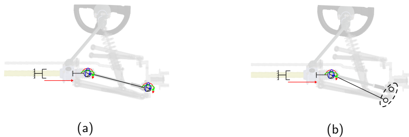
Figure 5.4: MB model of the left side of the steering system. The arrows represent the DOFs allowed by each joint. In 5.4a, the initial MB model is presented. Figure 5.4b shows the resulting MB model for the steering system after opening the closed-loops following the approach of the formulation selected in Section 3.2.
