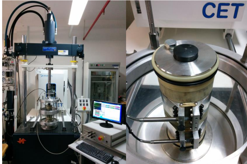
141 142 Fig. 2. Sample and sensor arrangement for resilient modulus triaxial test according to Standard EN 13286-7. 143
