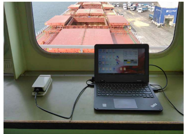
Fig. 4. IMU installed inside the vessel.
