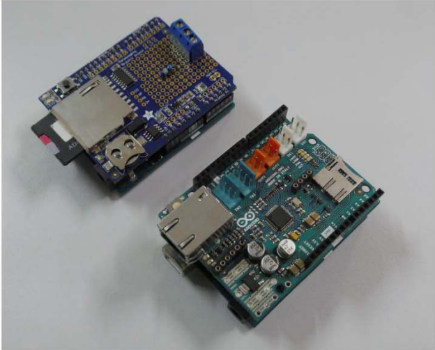
Figure 8. Arduino® datalogger and Ethernet board used to synchronize RTC chip.
