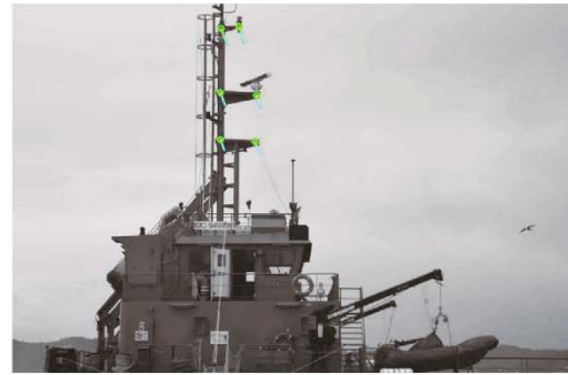
Fig. 12. Output of the stern camera during the assays. Selected features and corresponding displacement vectors are marked on the image.
