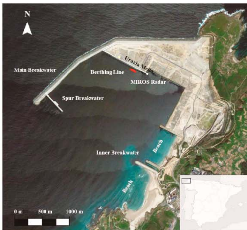
Fig. 9. Outer Port of A Coruña, in Punta Langosteira (Northwest of Spain), and mooring location of the Urania Mella during the assays, and location of the MIROS radar used to measure wave height.
