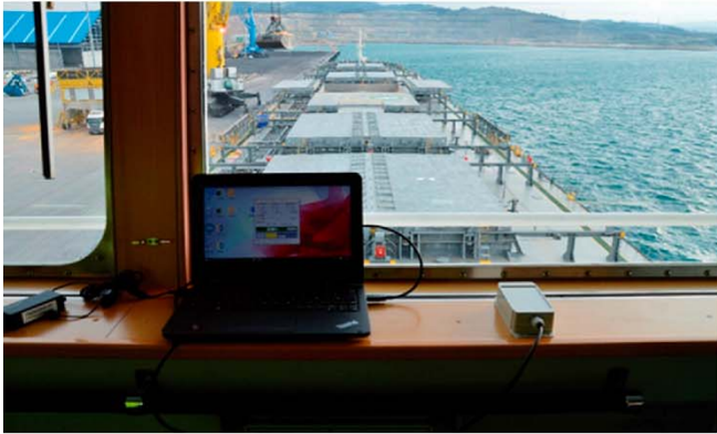
Figure 4. IMU installed inside of the vessel.
