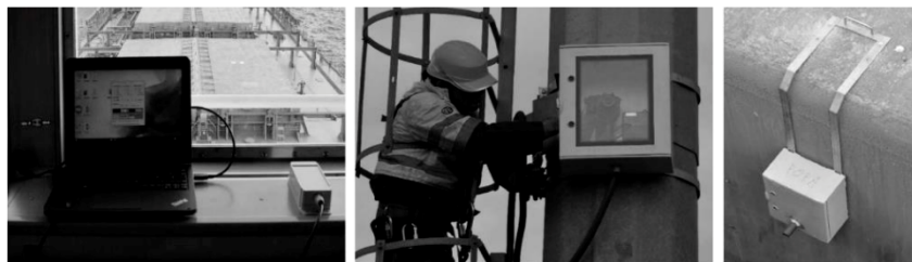
Figure 2. Left: IMU (Inertial measurement unit), Center: Photogrammetric techniques, Right: Laser distance sensor.
