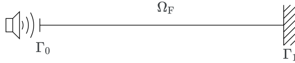
Figure 9: Diagram of the fluid model with speaker-rigid boundaries.
