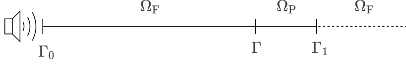
Figure 15: Diagram of the fluid-porous coupled model with speaker-transparent boundaries.
