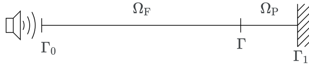
Figure 13: Diagram of the fluid-porous coupled model with speaker-rigid boundaries.
