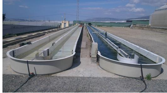
Figura 2: Fotobiorreactor industrial raceway
