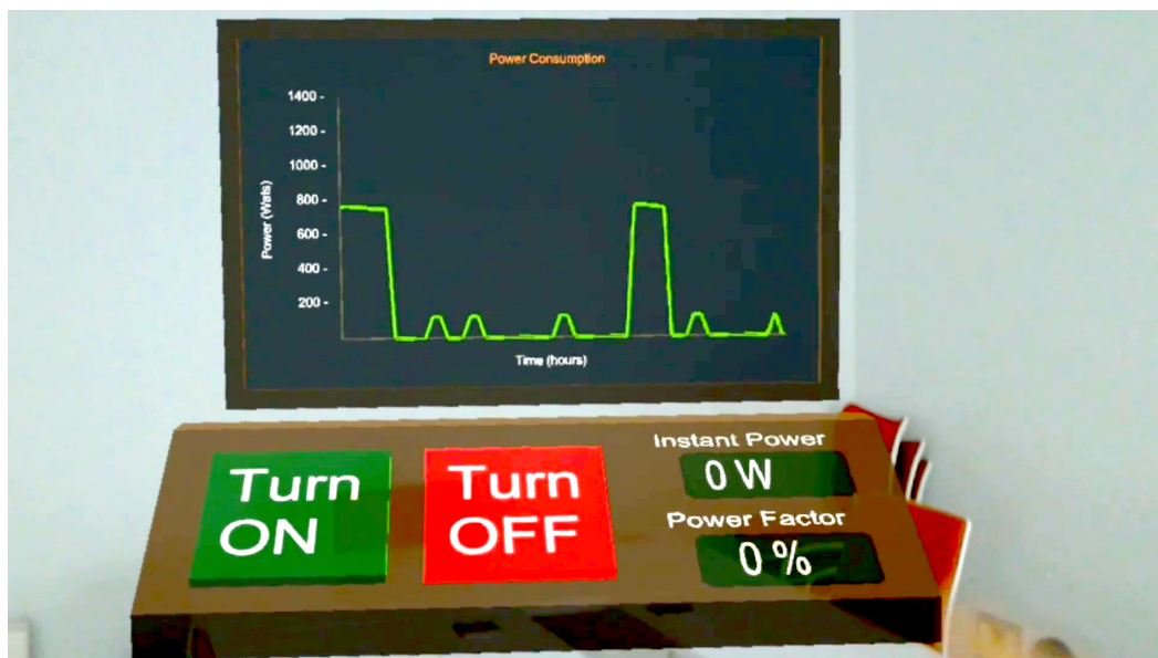
Figure 8. Virtual dashboard for controlling and monitoring the smart socket.
