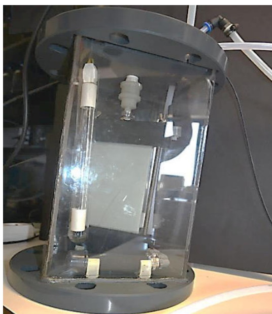
Figure 6.1 – Newly designed photocatalytic membrane reactor with submerged outside-inside flux membrane filtration system and UV lamps.
