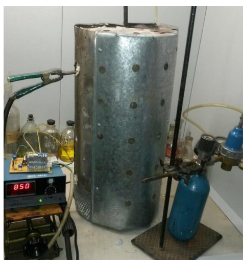
Figure 38. P4C activation setup: 1 - cylindrical electric furnace; 2 - reactor; 3 - thermocouple; 4 - argon (Ar) gas bottle; 5 - insulator; 6 - electric resistance heating.
