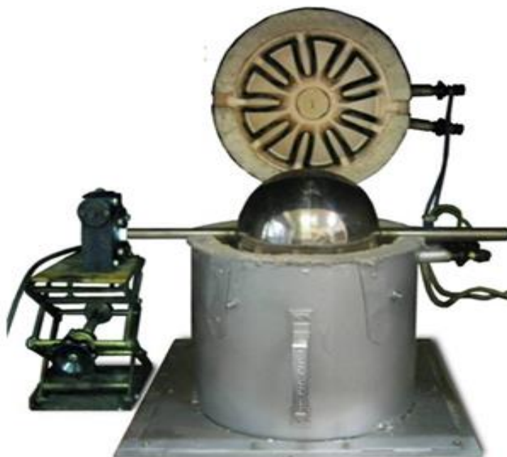
Figure 37. Spherical rotary steel reactor that originated P4C.
