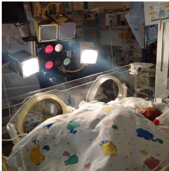
Figure 5.1: Experimental setup of the Neonaten dataset acquisitions. The cameras and dedicated light are installed in a tripod pointing at the neonate at a distance of approximately 1m.
