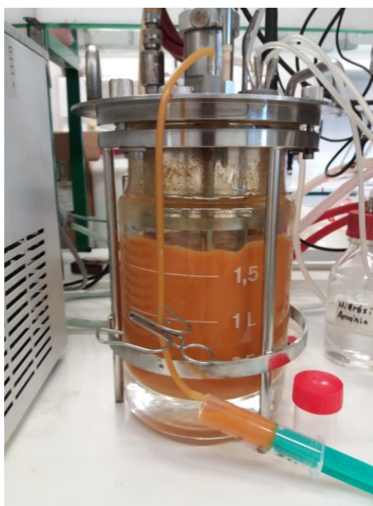
Figure 3.10 – Bioreactor with Pseudomonas chlororaphis subsp. aurantiaca DSM 19603 culture, during NH 4 OH -base assay, at 14 h fermentation.
