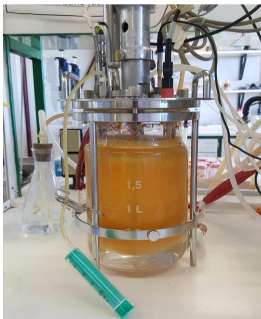
Figure 3.2 – Picture of the bioreactor with Pseudomonas chlororaphis subsp. aurantiaca DSM 19603 culture, during standard assay at 12 h fermentation.
