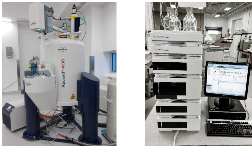
Figure 1.8 - Two of the analytical machines typically used in characterization of sophorolipids. Left: Bruker Avance III Ascend 400 MHz NMR Right: Agilent 1200 Series LC with Binary pump.
