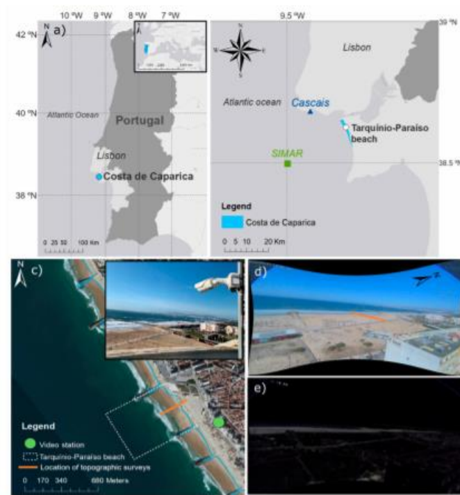
Figure 1. Study site map. (a) Location of Costa de Caparica; (b) location of Tarquinio-Paraiso beach (circle), Cascais tide gauge (triangle), and SIMAR point (square); (c) location of the video-station (in green) and of the cross-shore profile surveyed over the monitored period (orange, see Section 3.2); (d) Timex image and (e) Variance image.
