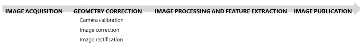
Figure 1. Major modules of a video-monitoring system (adapted from Taborda & Silva, 2012; Archetti et al., 2014)
