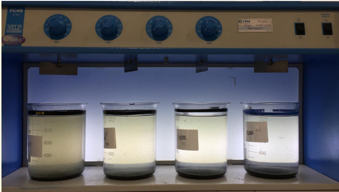
Figure 5.1-4: Jar tests with different doses of coagulant – after 20 minutes of sedimentation.
