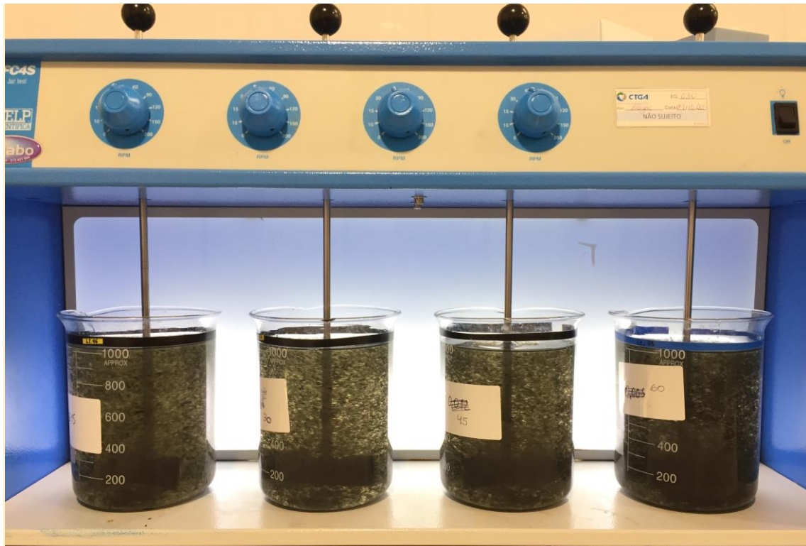
Figure 5.1-2: Jar tests with different doses of coagulant - beginning of the flocculation phase (slow mixing), post coagulation phase (rapid mixing).
