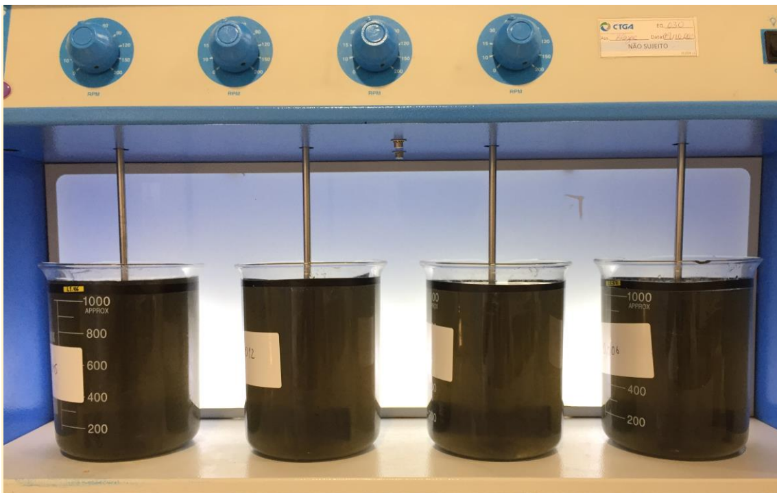
Figure 5.1-1: Four jars filled with raw wastewater from Espinho WWTP in the stirring machine where the Jar tests were performed.
