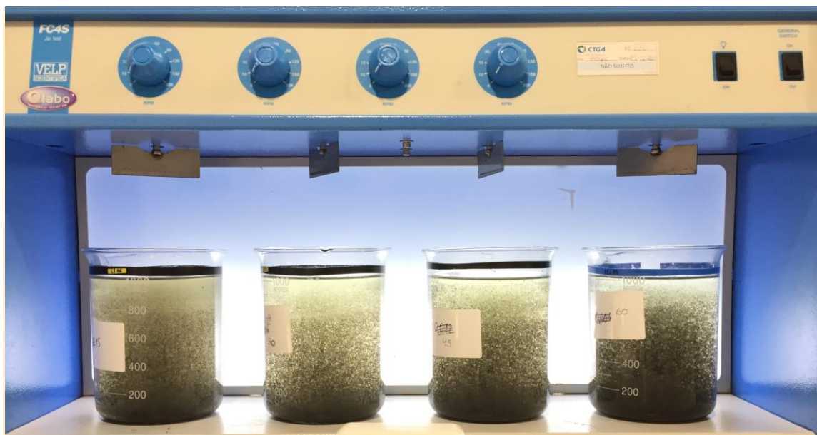
Figure 5.1-3: Jar tests with different doses of coagulant – beginning of the sedimentation phase.
