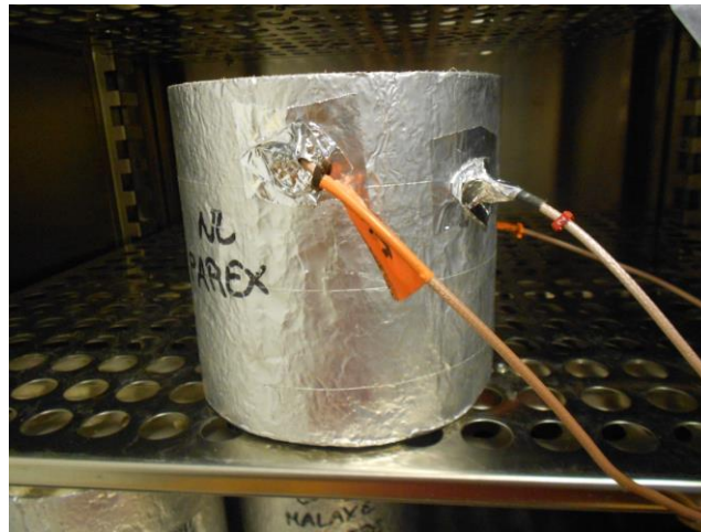
Figure 6.9- Prepared sample of NL in the climatic chamber
