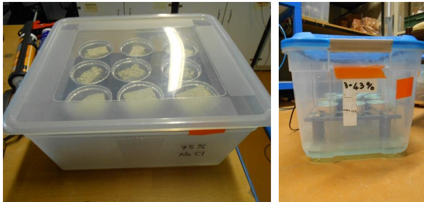
Figure 4.3- Sorption isotherms setup (Left- procedure at 40°C and Right- procedure at 23°C)
