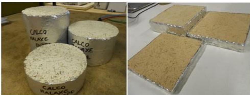
Figure 4.6- Example of samples for Moisture buffering test (Left- Hemp concrete Calco; Right- Earth mortar plaster F3)
