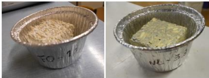
Figure 4.2- Samples setup for sorption isotherms test (Left- Earth mortar plaster F0; Right- Hemp concrete NL)
