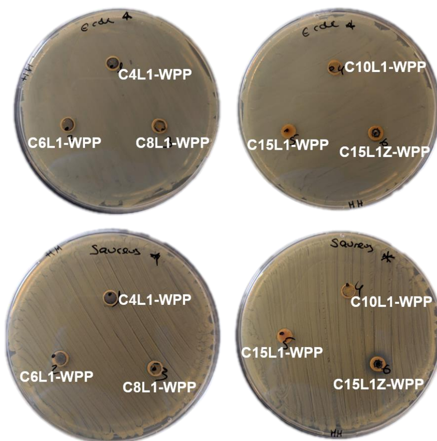
Figure 3.8 - Wells filled with cork WPP samples (Table B. 2). Top row: Samples in a culture with E. coli bacteria; Bottom row: Samples in a culture with S. aureus bacteria.
