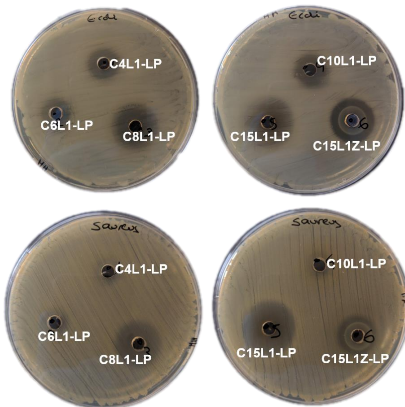
Figure 3.6 - Wells filled with cork LP samples (Table B. 2). Top row: Samples in a culture with E. coli bacteria; Bottom row: Samples in a culture with S. aureus bacteria.
