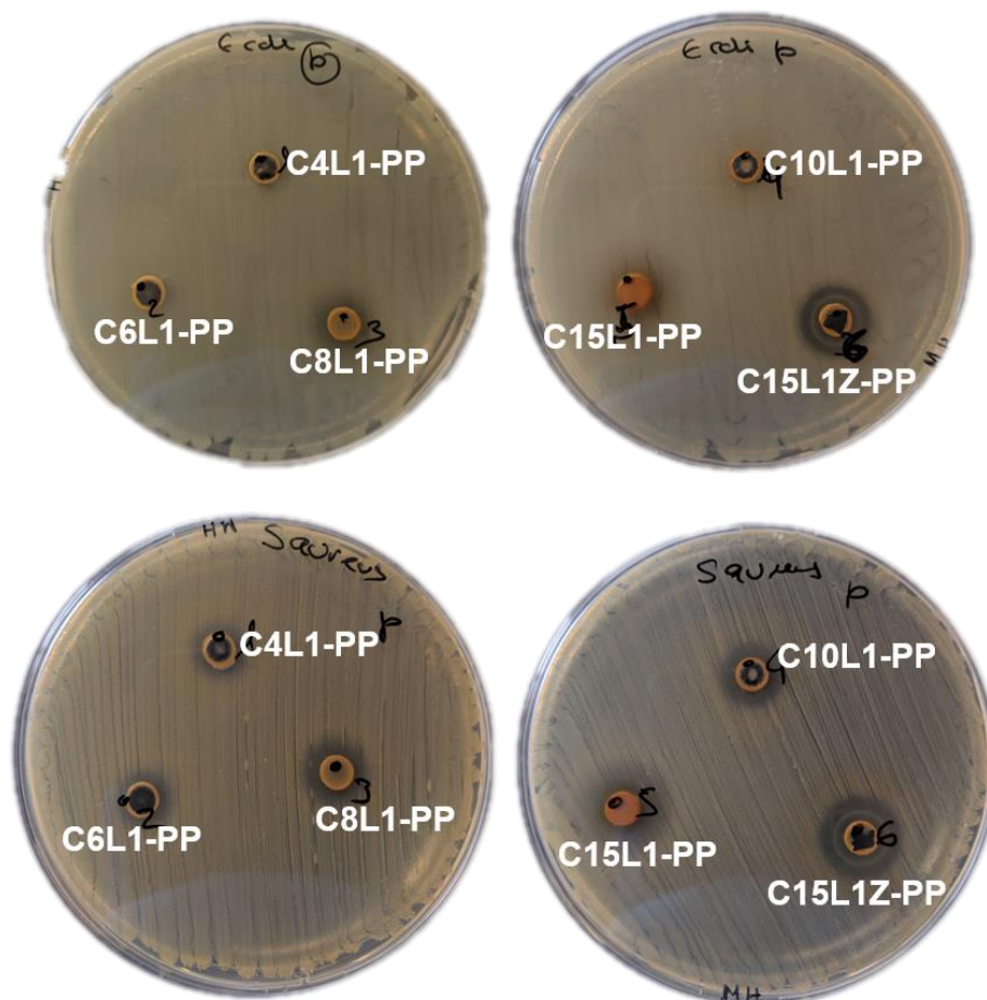
Figure 3.7 - Wells filled with cork PP samples (Table B. 2). Top row: Samples in a culture with E. coli bacteria; Bottom row: Samples in a culture with S. aureus bacteria.
