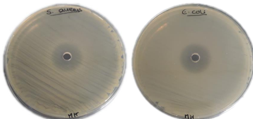
Figure 3.5 – Wells filled with solvent system (LiOH/Urea/H 2 O – 4.6:15:80.4 wt. %) as a reference sample for both bacteria's ( S.aureus at left and E.coli at right).
