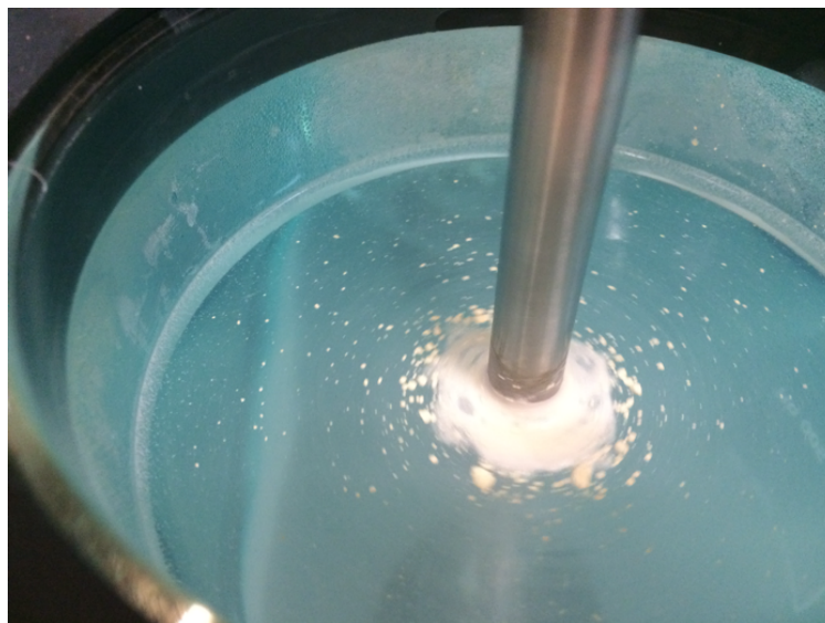
Figure 3.16 – Floating powder during ITZ SDD dissolution testing.
