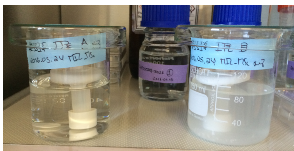
Figure 3.3 – ITZ dissolution and permeation experiment in FeSSIF. On the left, ITZ is available as a compressed pellet, on the right ITZ is available as a powder.
