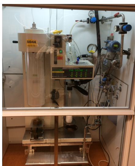
Figure 3.4 – SDD production in a Buchi Mini Spray Dryer B-290.
