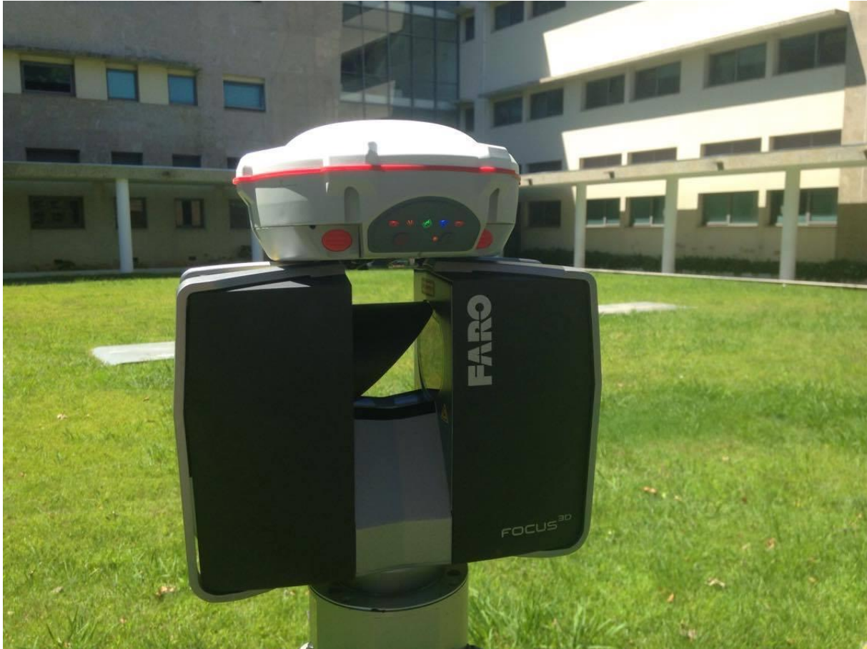
Figure 13 Shows the work of the receiver which is set on the FARO Laser
