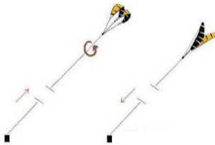
Figure 2.4 - Rotokite operation principal [13]
