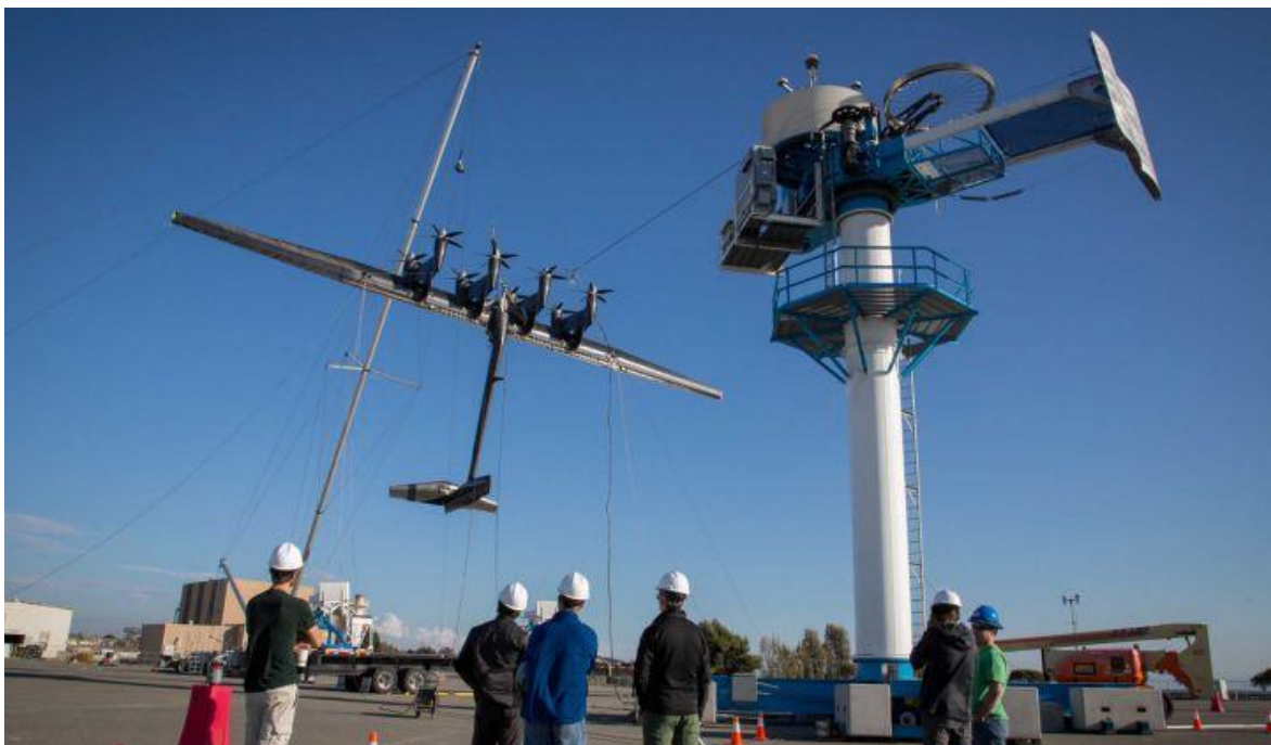
Figure 2.24 - Makani kite commissioning [20]
