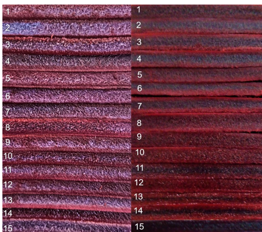
Figure 31 - Pile of the cattle the samples submitted to the Sudan IV staining test before (on the left) and after (on the right) drying for visual comparison.
