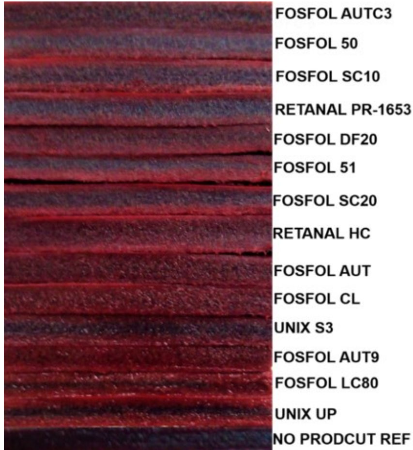
Figure 17 - Pile of all the mechanically dried cattle samples submitted to the Sudan IV staining test for visual comparison.
