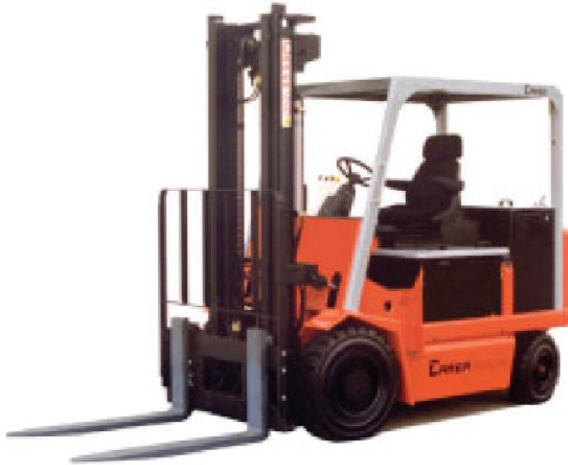
Figure 5.1 – Carer R45NCF electric forklift [Carer2019]
