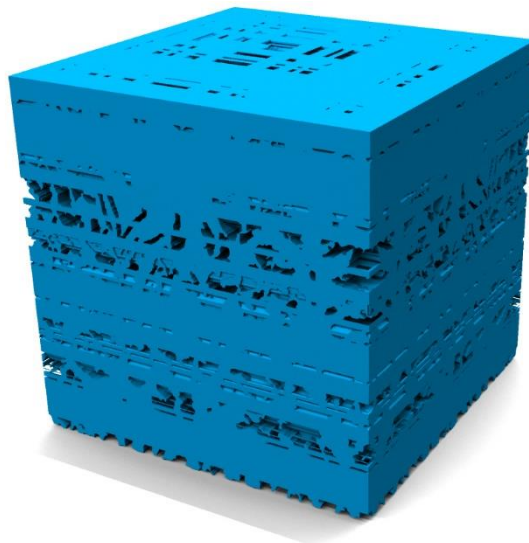
Figure 3.20 – Electrolyte volume from electrode porosity modelling
