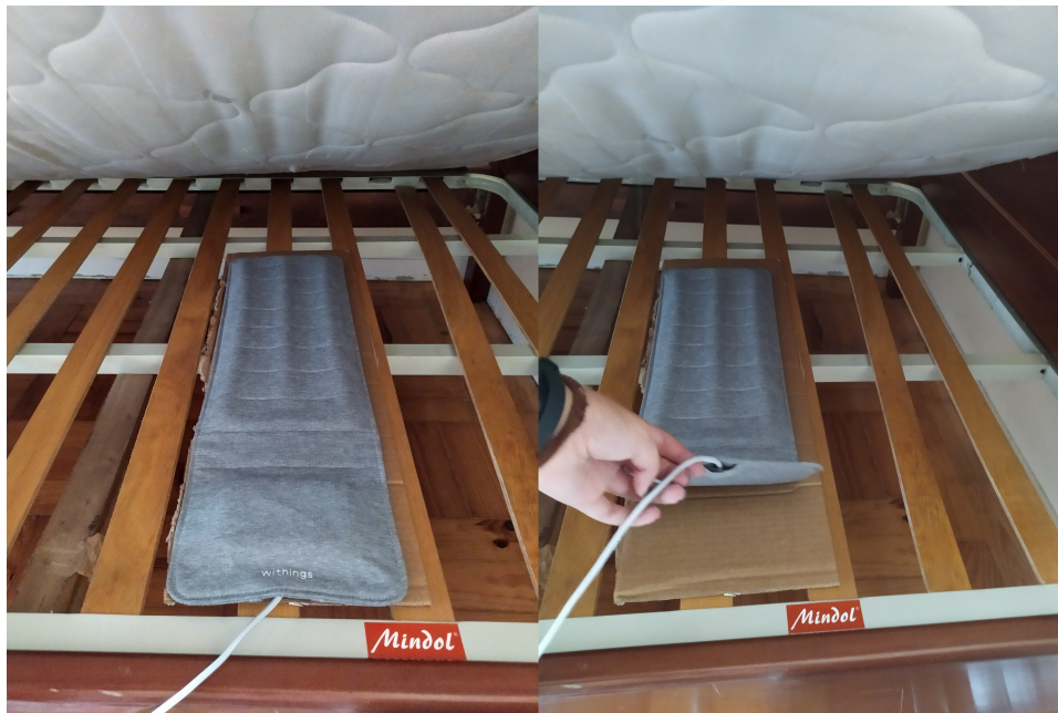
Figure 4.2: Photos of the sensor placed during the experiment. The sensor needs a sturdy surface to be on, so it was placed cardboard over the bed frame. The sensor is in contact with a spring mattress.
