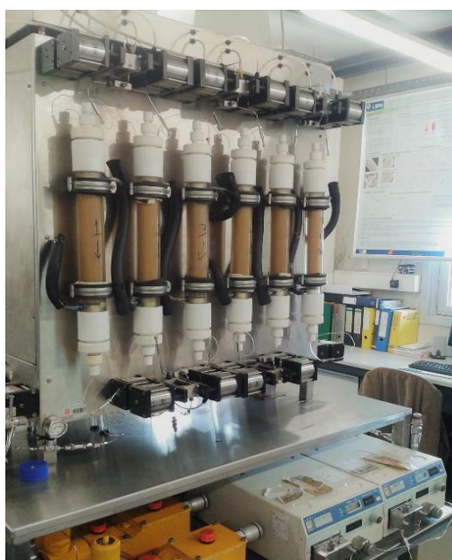
Figure 5.2. SMBR LICOSEP pilot scale unit with 12 columns (a side view with 6 columns).
