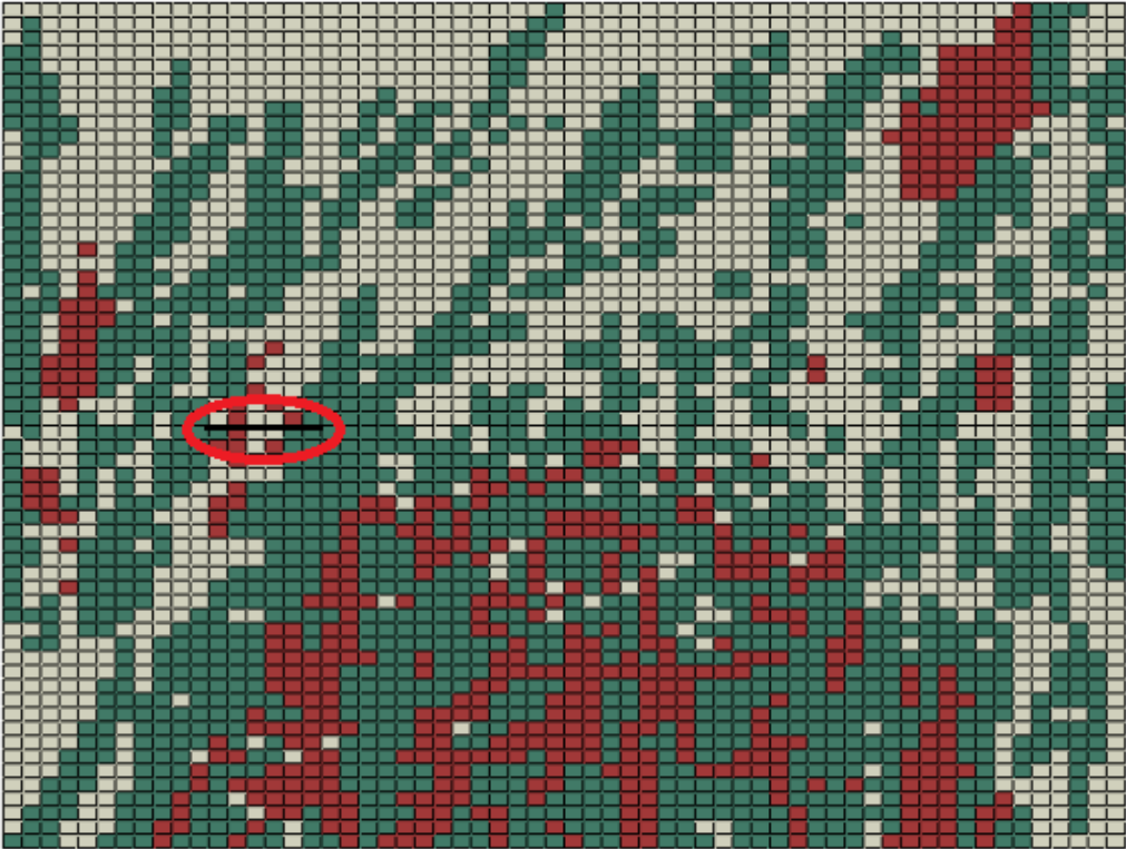
Figure 5.6 Microstructure Mesh cooling rate 7.2°Cmin-1, Horizontal Crack Region A, 60 nm
