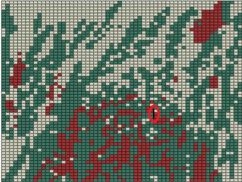
Figure 5.7 Microstructure Mesh cooling rate 7.2°Cmin-1, Vertical crack
