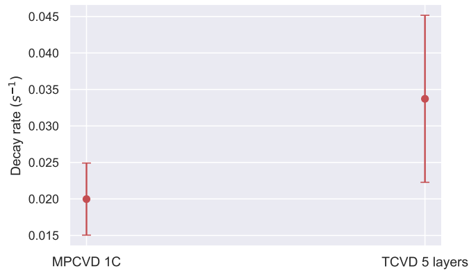
FIGURE 3.20: Decay rate for the MPCVD-grown 1C and the 5 layers TCVD-grown graphene sample
