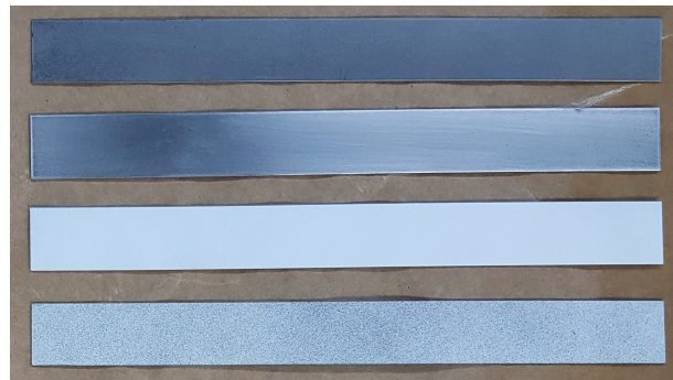
Figure 3.5: Specimen preparation for r-value measurement using DIC.
