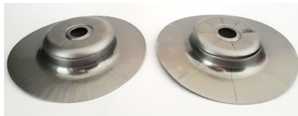
Figure 3.40: Fracture experimental cases when the critical blank diameter was exceeded (DP780 using the blank diameters of 135 mm and 130 mm, left to right, respectively).
