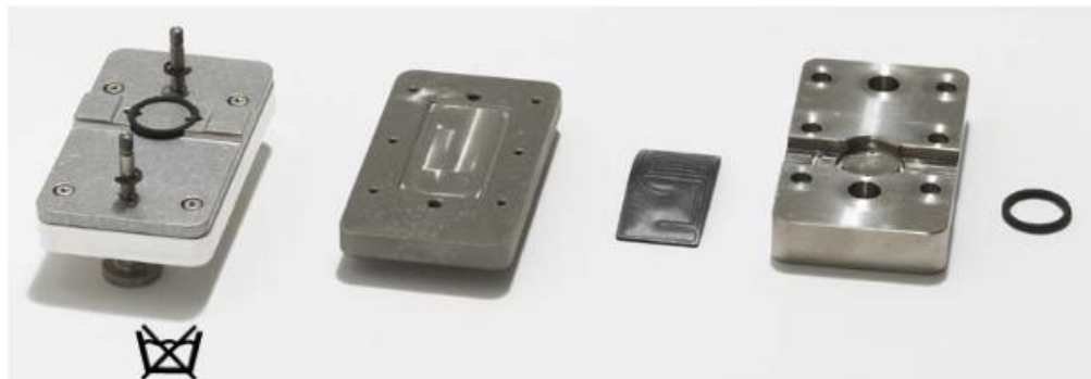
Figure 6. Different parts of the flow module disassembled for cleaning. (Q-Sense, 2008).
