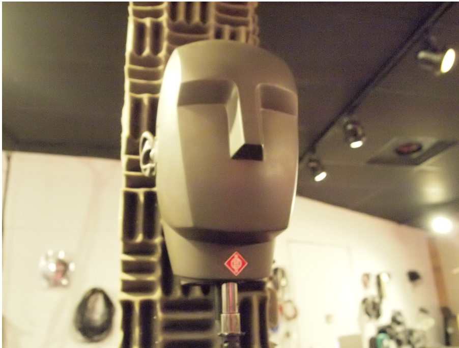
Figure 2.16: Neumann Ku 100 used for binaural recording ( Georg Neumann Ku 100 Dummy Head , 2011)
