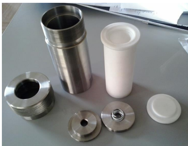
Figure 2.1. Teflon stainless-steel autoclave for hydrothermal synthesis.
