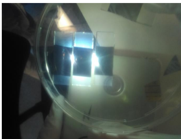
Figure 8.3. FTO with Fe thin film deposited by ion beam deposition, showing against-light a homogeneous deposition.
