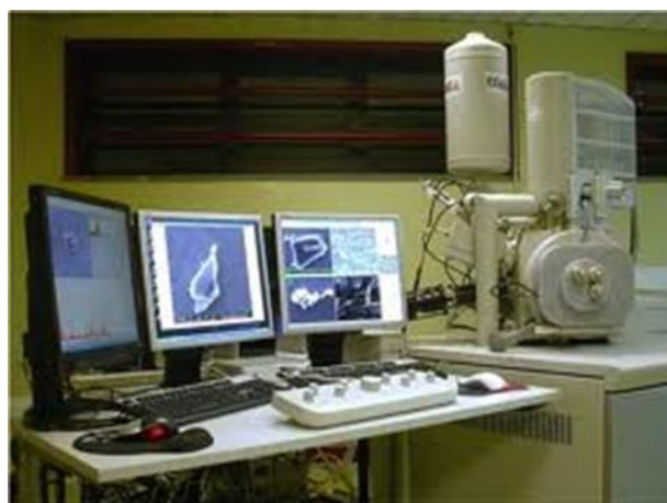
Figure 2.7. Scanning Electron Microscope, model Quanta 400FEG ESEM/EDAX Genesis X4M, at the CEMUP center from University of Porto (Extracted from [229]).
