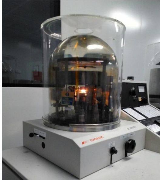
Figure 2.3. Electron-beam evaporation system used for Fe thin films deposition.
