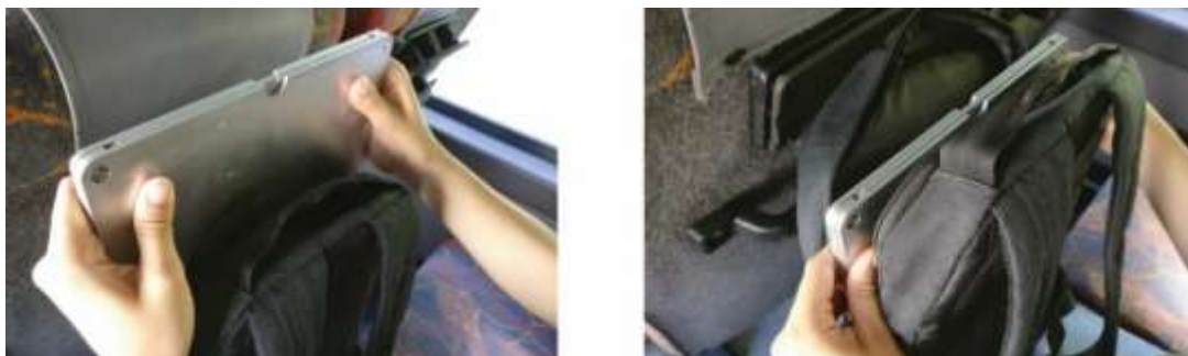
Figure 98: Placing the prototype of the lapdesk in a 15.6in laptop backpack to check if it fits.
