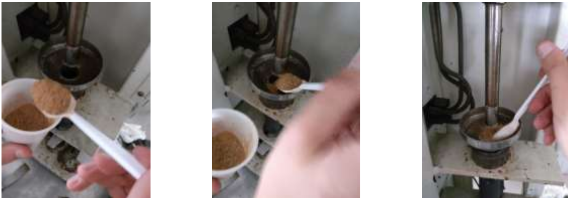
Figure 56: Process of cleaning the cylinder of the injection machine.
