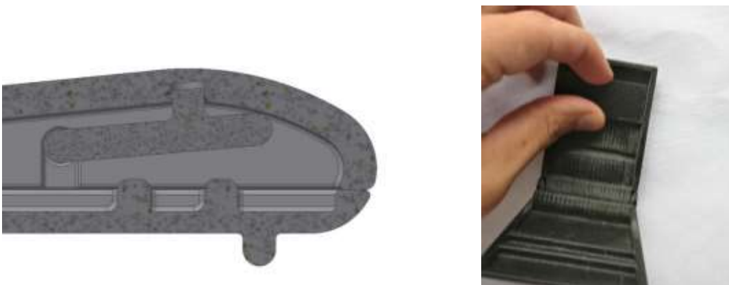
Figure 90: Representation of how part C gets fixed and trying to pull part C from the fixed position.
