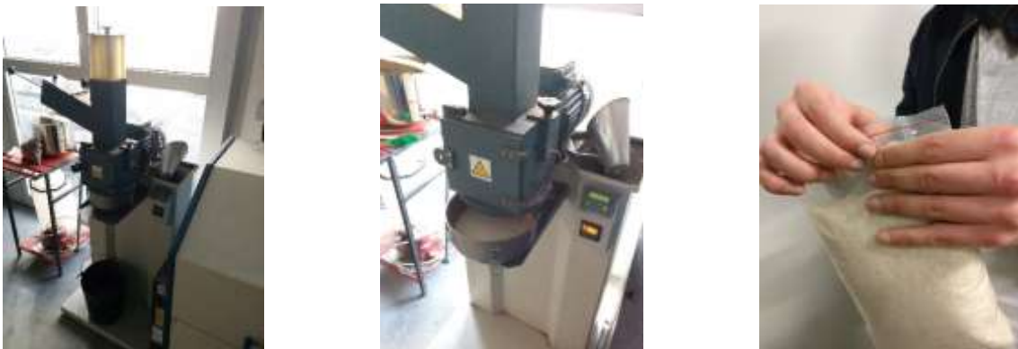
Figure 41: Process of grinding the PLA in a grinder in the Laboratory of the DEMM.
