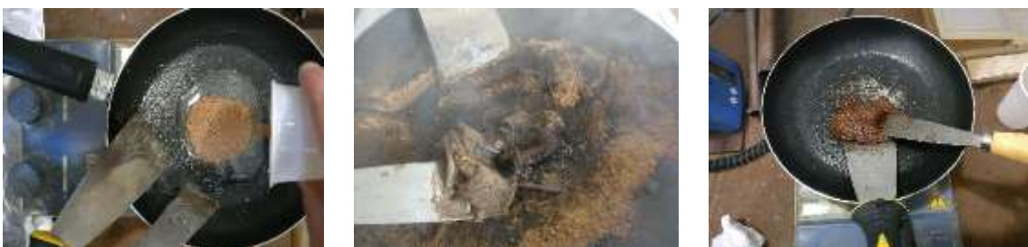
Figure 44: Blending the melted PLA with the almond by-products particles.
