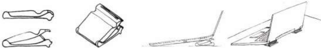
Figure 2. Concept design of the laptop stand using the composite PLA + almond by-products.
