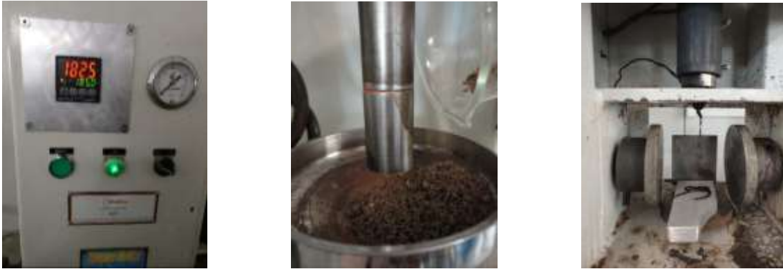
Figure 51: Placement of material in the cylinder to eliminate any residues of other polymers.
