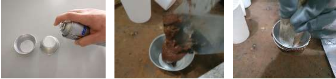
Figure 57: Step g – Process of placing the melted material in the aluminium cupcake mould, which was previously sprayed with a release agent spray, and hand pressure with the help of a stick to avoid burning in the hands.
