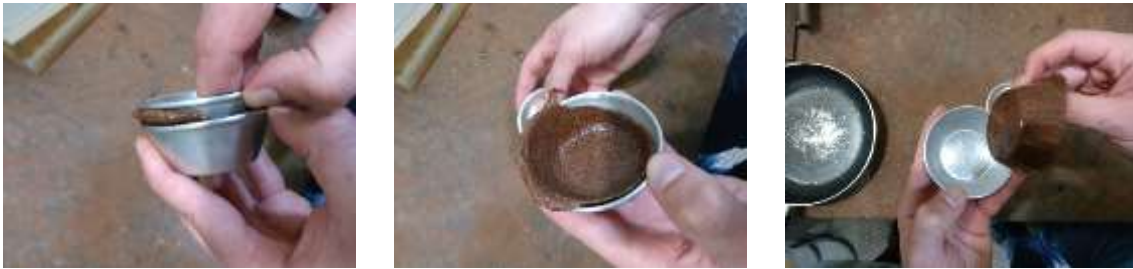
Figure 58: Step h – Process of removing the piece from the aluminium cupcake mould.
