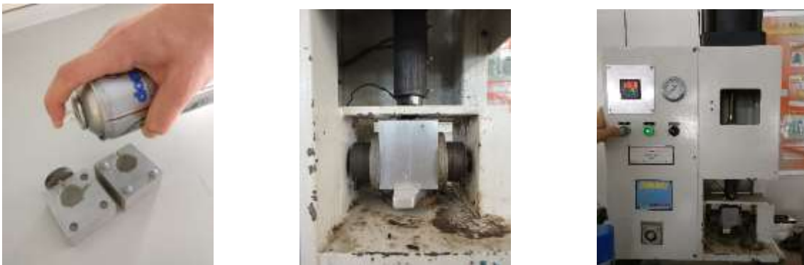
Figure 52: Preparing the mould for an injection.
