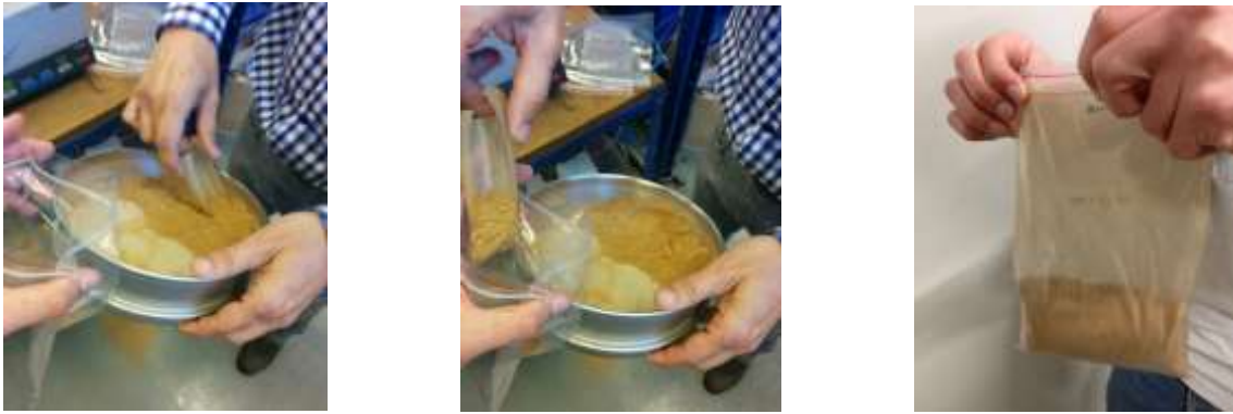
Figure 39: Process of separating the sieved particles into plastic zip bags by particle-size distribution in INEGI.
