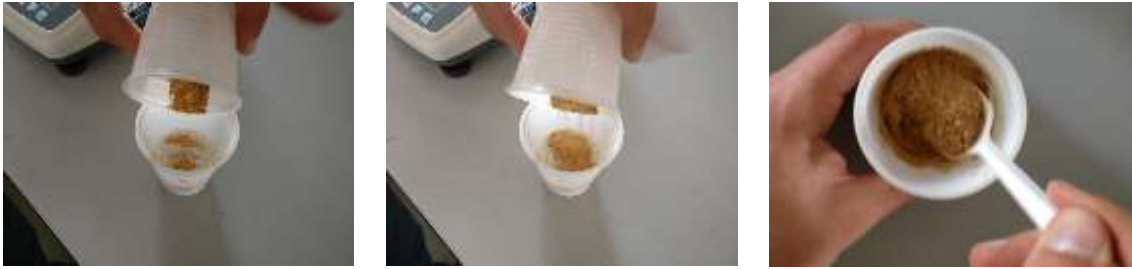
Figure 55: Mixing grinded PLA with the almond by-products particles.
