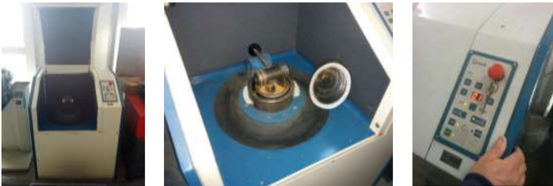
Figure 37: Process of milling the grinded almond by-products in a vibratory disc miller in the Laboratory of the DEMM.
