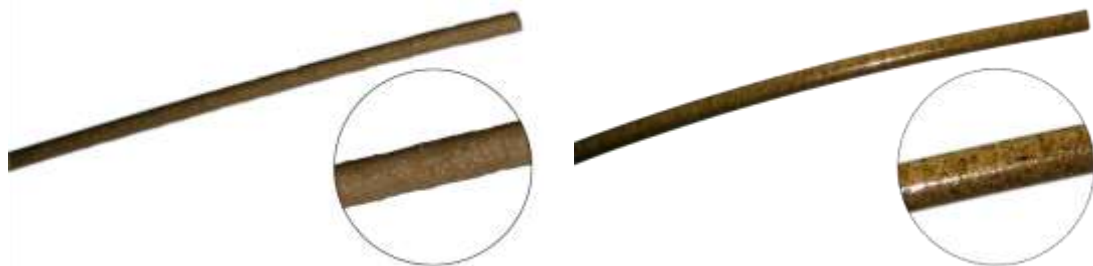
Figure 61: 3D printing wires – PLA + wood fibres on the left, and PLA + coffee particles on the right.
