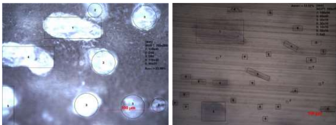
Figure 66: Example of how it was calculated the percentage of reinforcement in each wire – WWF on the left and WCP on the right.
