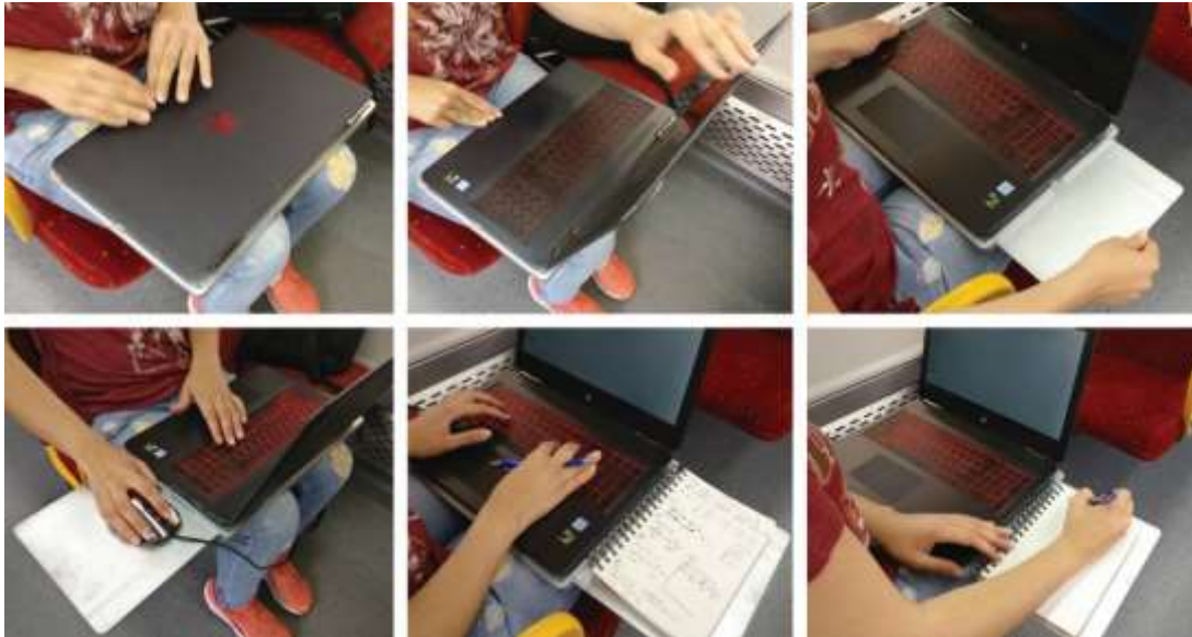
Figure 100: The user testing the sliding surface both for the mouse and to write on a book.
