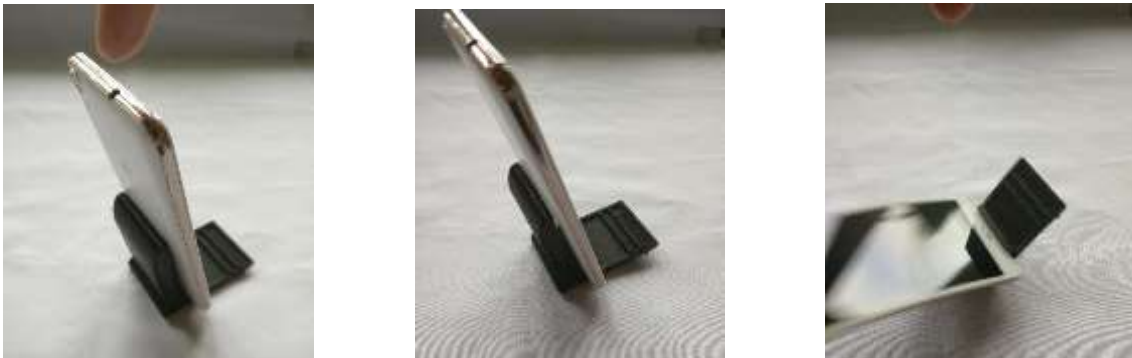
Figure 89: Applying a small force in the top of the smartphone, it will easily topple.
