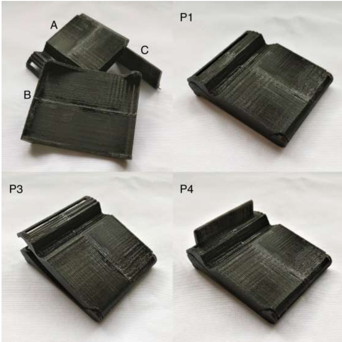
Figure 80: Prototype, using a FDM 3D printer, of the three parts and respective assembling with configurations P1 , P3 and P4 .
