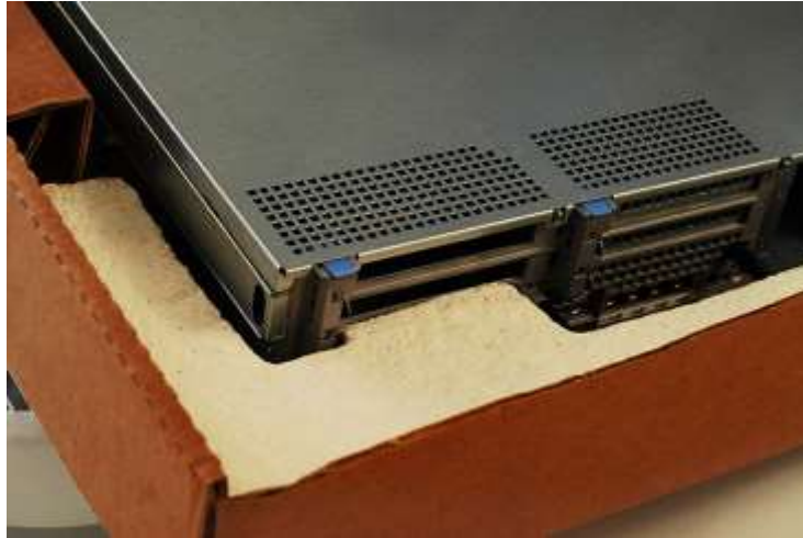
Figure 22: MycoFoam™ application: Mushroom® Packaging components that provide cushioning and bracing in large packages for Dell servers (Ecovative Design).
