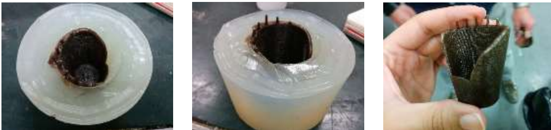
Figure 48: Removing the coffee cup with 5% of reinforcement from the silicone mould.
