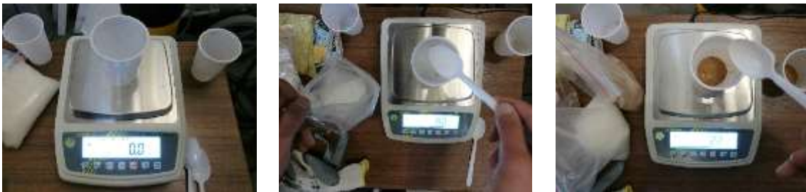
Figure 42: Measuring the weight of the PLA and almond by-product particles before being blended.
