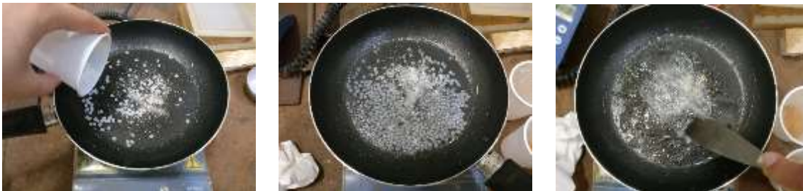
Figure 43: Melting the PLA pellets in a frying pan.
