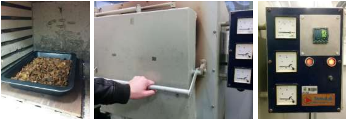
Figure 35: Process of removing part of the moisture from the almond by-products by placing them in a furnace, for 12h at 80°C, in the Heat Treatment Laboratory.
