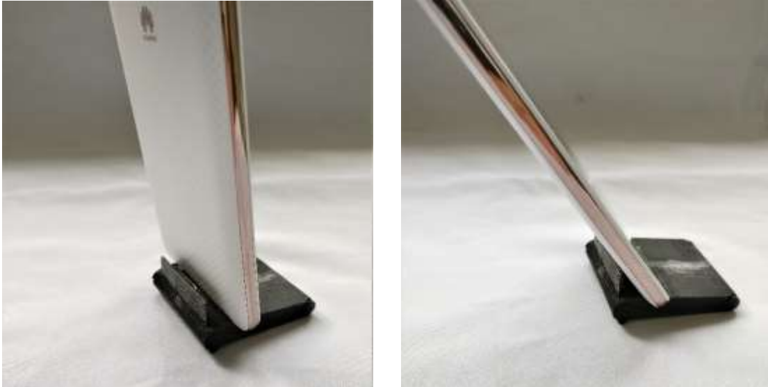
Figure 81: The multifunctional stand cannot prevent smartphones or tablets from toppling.
