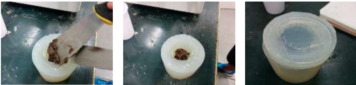
Figure 47: Creating a coffee cup by hand pressure using a silicone mould.
