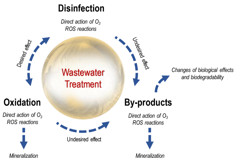
Figure 2.6. Main goals for the application of ozone. Both processes are accompanied by the undesired formation of by-products (adapted from [195, 227]).
