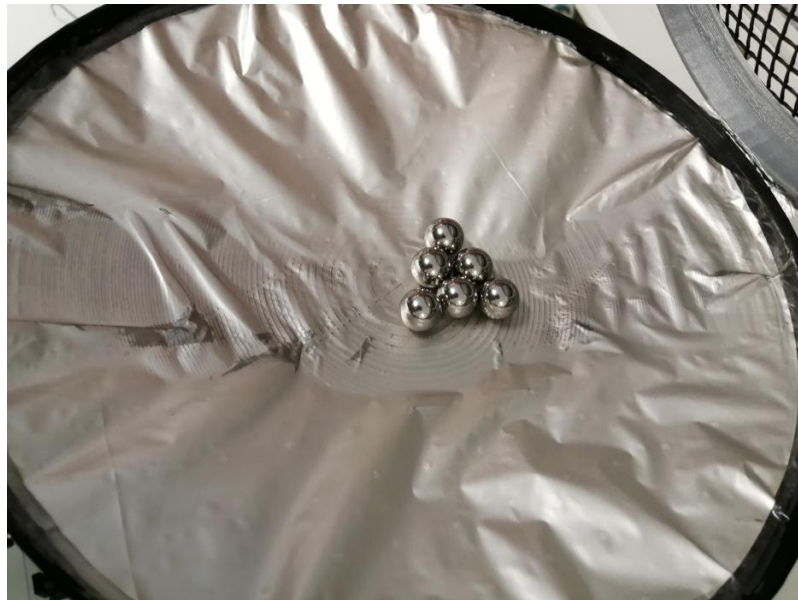
FIGURE 5.4: State of the ISOTENG after the degradation test.
