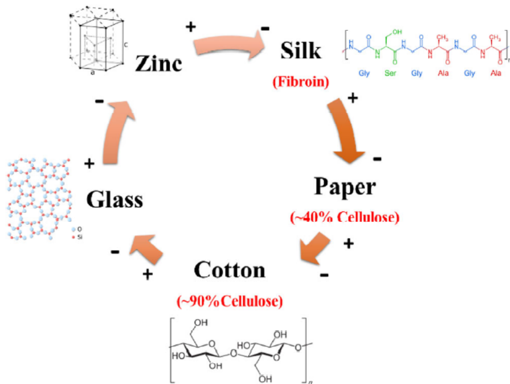
FIGURE 2.3: Example of a cyclic triboelectric series [12].
