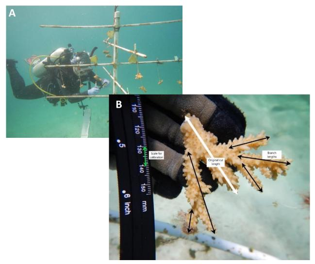
**Figure 8**. A) Data collection, and B) Example of TLE calculation done in the field or Image J, if applicable. Highlighted are the original cut length, branch lengths, and scale used in Image J for calibration.
