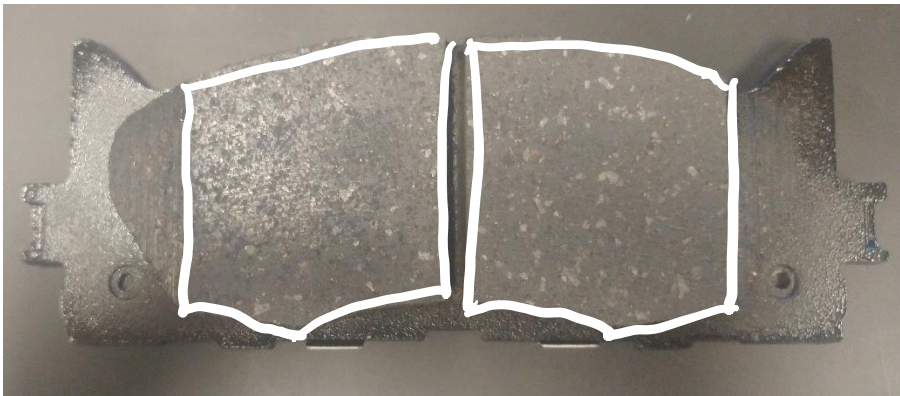
Figure 3: Apparent contact area of one Akebono brake pad (there are 2 used in the full scale dynamometer)
