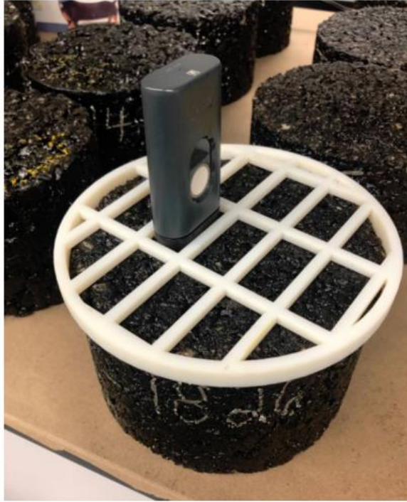
Figure 4-2. The 3D printed mold used for scanning asphalt mixture samples
