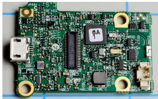
Figure 2-5. Main board used in the sensor
