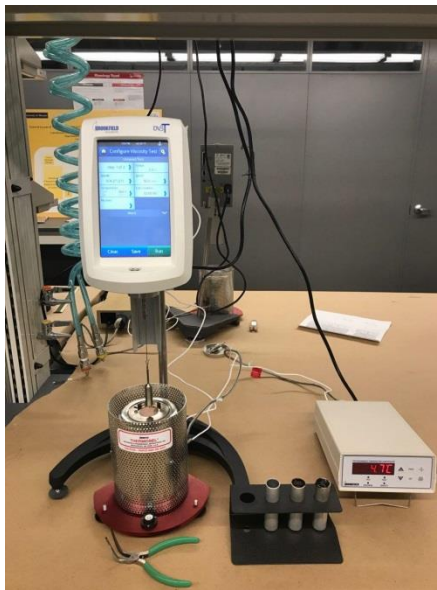
Figure 2-9. RV device and details of its displaying monitor
