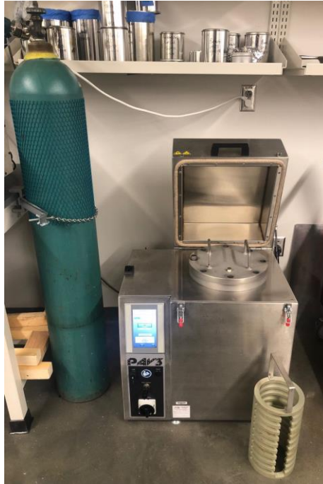
Figure 2-8. Pressure aging vessel (PAV) apparatus at MAPIL
