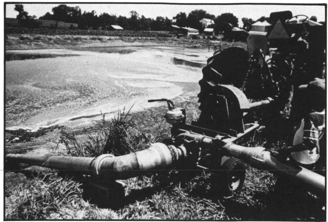
Figure 10. Tractor-powered PTO pumps are commonly used to pump lagoon effluent.
