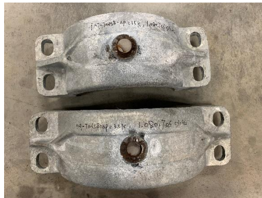
Figure 44. Failure of FAT-TENS8 Tested at 5.8 ksi
