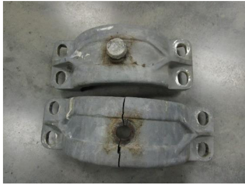
(a) Failure of FAT-TENS(USED)2
