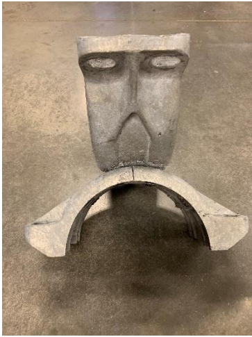
(a) Crack on One Side Cut Through the Thickness
