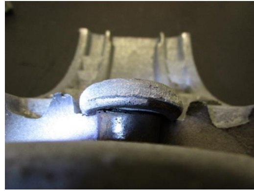
(b) Rivet Cracking
