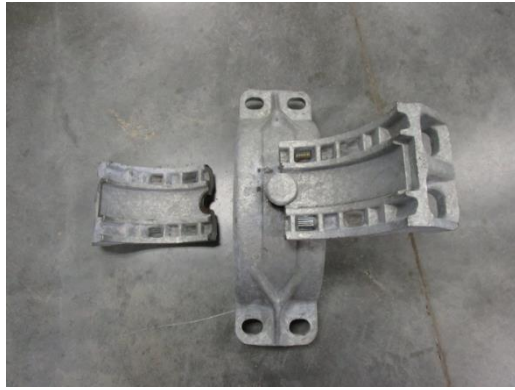
(a) Coupler Cracking
