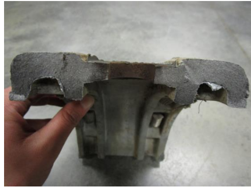
(b) Failure Surface of FAT-TENS(USED)2
