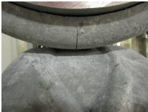
(a) Crack at 7,214,300 Cycles
