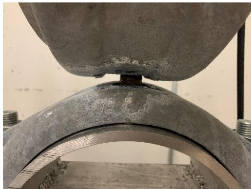
(a) Failure of FAT-TENS7
