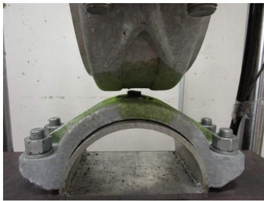
(a) Rivet Cracking
