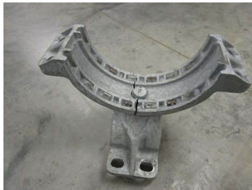
Figure 38. Failure of FAT-TENS4 Tested at 5.8 ksi
