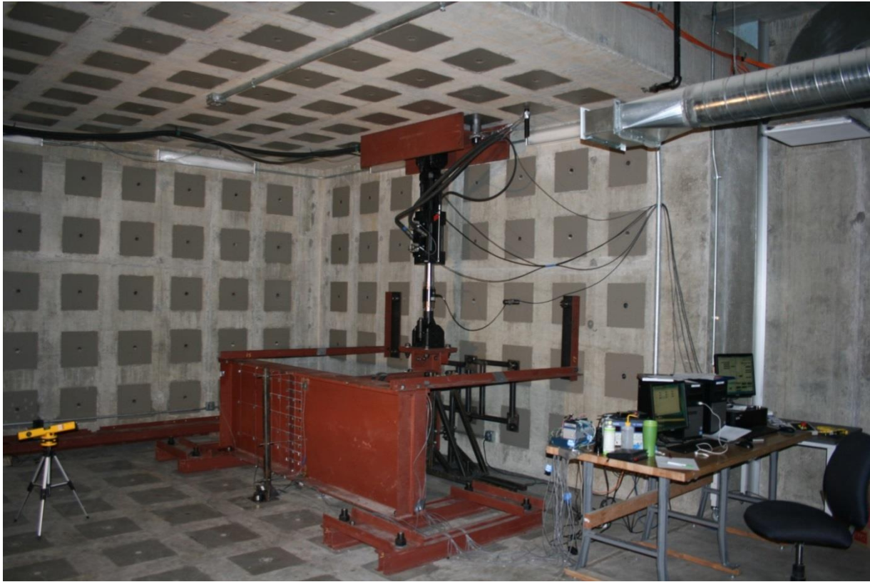
Figure 2 Girder subassembly 2 being tested at the Fatigue and Fracture Laboratory.
