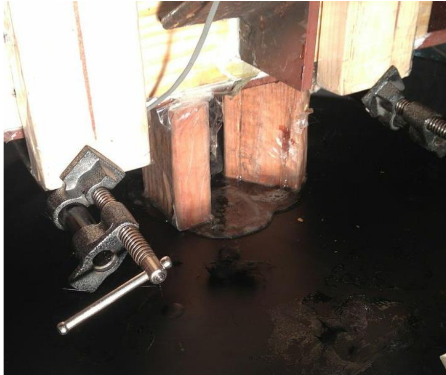
Figure B 6: Epoxy leaking out of mold insuring air pockets wouldn't be present in the block
