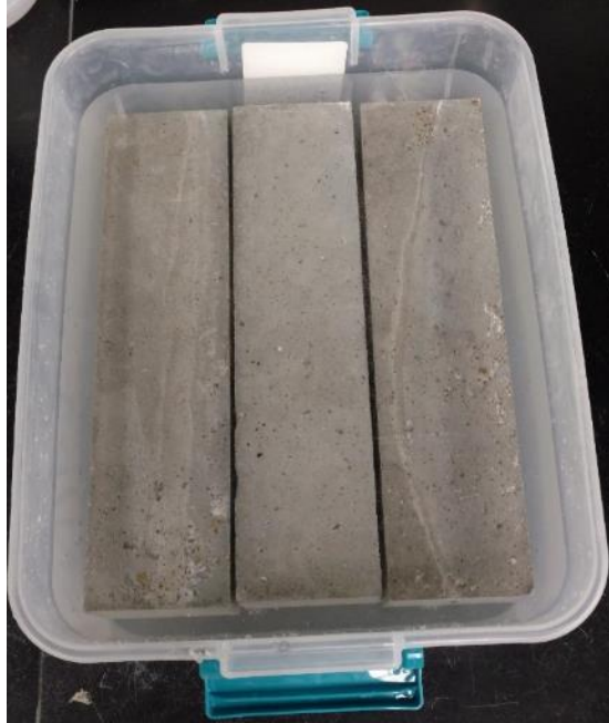
Figure 2.3: Concrete specimens (wetting phase)
