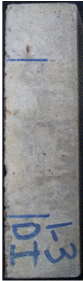
(a) Control (100% portland cement, 0% fly ash)
