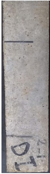
(a) Control (100% portland cement, 0% fly ash)
