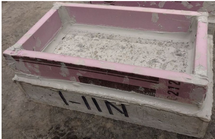
Figure 3.1: Scaling resistance test specimen
