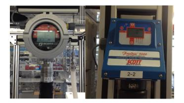
**Figure 7.3.** Ammonia Gas monitors (a) Scott Meridian Detector with Ammonia Sensor located in the ventilated enclosure (b) Freedom 5000 Detector with Ammonia Sensor located in the laboratory
