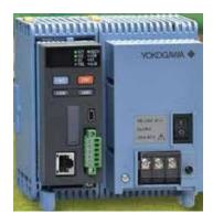
**Figure 7.4**. Yokogawa Data Acquisition Unit to monitor the NH<sub>3</sub> concentration in the ventilated enclosure and the laboratory
