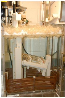
**Figure 2.8**. Liquid-Liquid Equilibria Apparatus. Picture in the left show experimental apparatus, tubes, and cathotemeter. The picture in the left demonstrates the mixing of the borosilicate tubes via the rocking movement. *This picture was taken at DuPont Experimental Station, Wilmington, Delaware, and used in this thesis with the permission of Dr. Mark B. Shiflett.*
