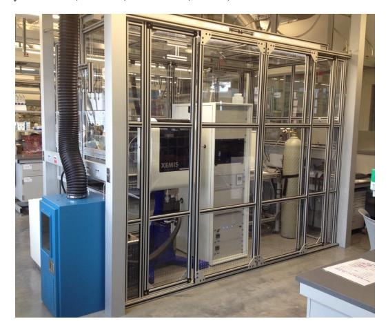
Figure 2.1. XEMIS Microbalance in a ventilated enclosure at the University of Kansas
