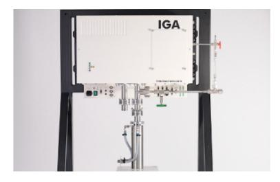
Figure 2.5. Intelligent Gravimetric Analyzer (IGA) Microbalance <sup>74</sup>
