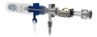
Figure 2.4. The XEMIS microbalance beam view.<sup>72</sup>
