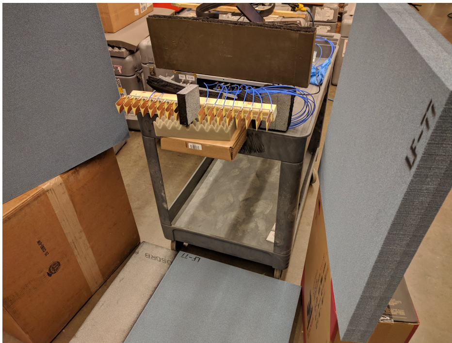
Figure D.2: Photo of the placement of RF absorbing foam around the radar
