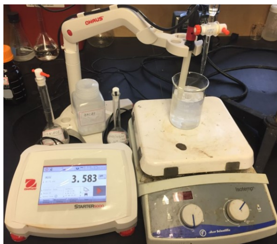
Figure 3.9: Titration for aldehyde group content determination.
