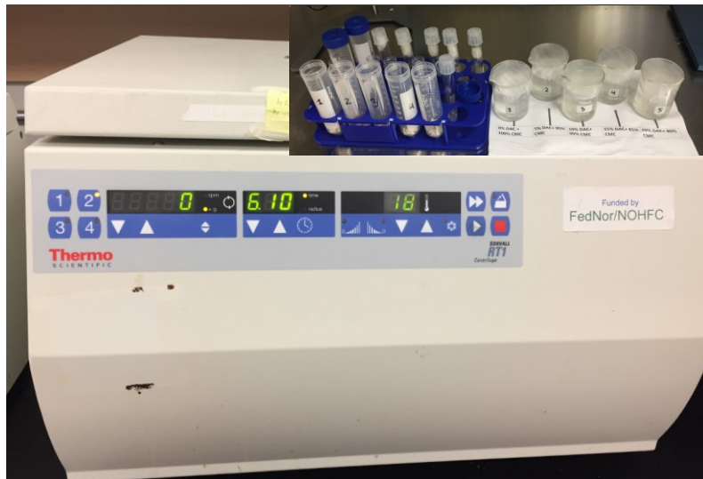
Figure 3.10: Sorvall RT1 Centrifuge for water uptake calculations.
