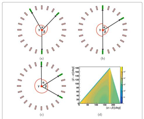
**Fig. 6 a–c** The three cases based on the angular correlation between the 3 hits in an event. The origin of the visualized events is explained in the text. **a** The case when the sum of two smallest angles is greater than 180°. **b** The case when sum is 180°. **c** When the sum of two smallest angles is less than 180°. **d** The measured scatter plot of the difference  $(\beta - \alpha)$  vs the sum  $(\alpha + \beta)$  of the two smallest angles
