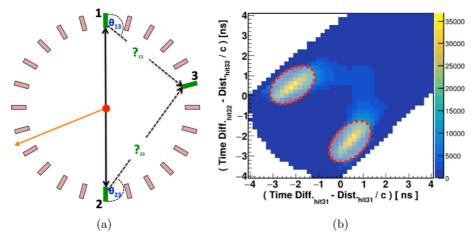
**Fig. 7 a** Pictorial representation of the event selection based on the algorithm used to tag the 511 keV photons. **b** The encircled dotted red lines show the selected scattering events of back-to-back photons based on the scatter test **S**
