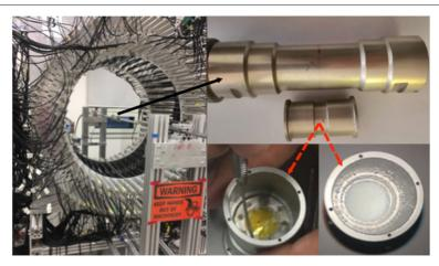
**Fig. 3** Experimental set-up of the annihilation chamber with the source placed at the center of the J-PET tomograph
