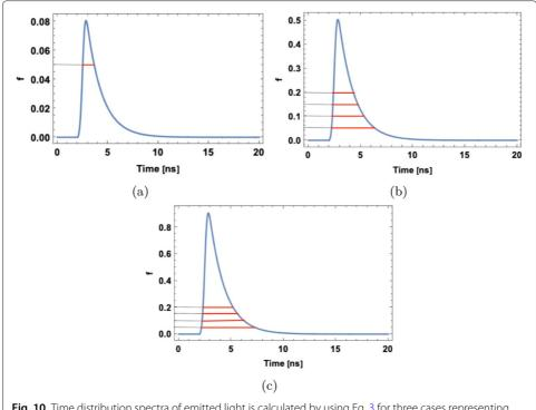
**Fig. 10** Time distribution spectra of emitted light is calculated by using Eq. 3 for three cases representing signals corresponding to the energy deposition of 80 keV (**a**), 500 keV (**b**), and 900 keV (**c**)
