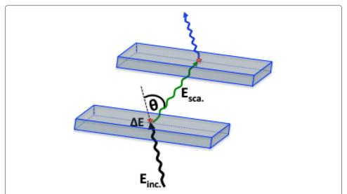
**Fig. 5** The incoming and scattered photon interactions are presented with two exemplary scintillators. Knowing the positions of emission of  $E_{inc}$  photon and positions of interactions of  $E_{inc}$  and  $E_{sca}$  photons inside the scintillators allow to estimate the scattering angle
