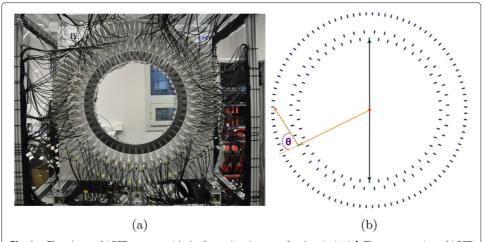
**Fig. 1 a** The photo of J-PET scanner with the front view (see text for description). **b** The cross section of J-PET with superimposed arrows depicting the interaction of 511 keV photons (black solid arrows) originating from positron-electron annihilation and prompt photon 1275 keV before (orange solid arrow) and after (orange dashed arrow) scattering inside the scintillator. Red dot in the center represents the <sup>22</sup>Na source
