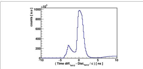
**Fig. 9** Results of the **S**-test calculated between hit 1 and hit 2 in event-wise manner. For the true scattering of prompt photons, the value of the S test is chosen between -0.5 and 0.75 ns. Small peak around S = -3 ns is mainly due to the contribution from back-to-back annihilation photons. A slope starting at 5 ns is because of the time difference constraint between hit 1 and hit 3 (> 10 ns)
