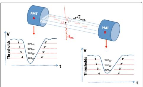
**Fig. 2** Illustration of the analog signals obtained at photomultipliers as the outcome of the energy deposited by the photon in the interaction with plastic scintillator. Each signal is probed at four fixed thresholds. The TOT value is calculated at each pre-defined voltage threshold, and the sum of all four TOT values from both photomultipliers (PMTs) gives the final TOT value, Eq. 1
