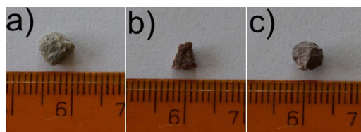
Fig. 1. Samples of the Rotliegend sandstones extracted from borehole CG5 at depth of (a) 2679.6 m, (b) 2741.4 m, (c) 2742.4 m.
