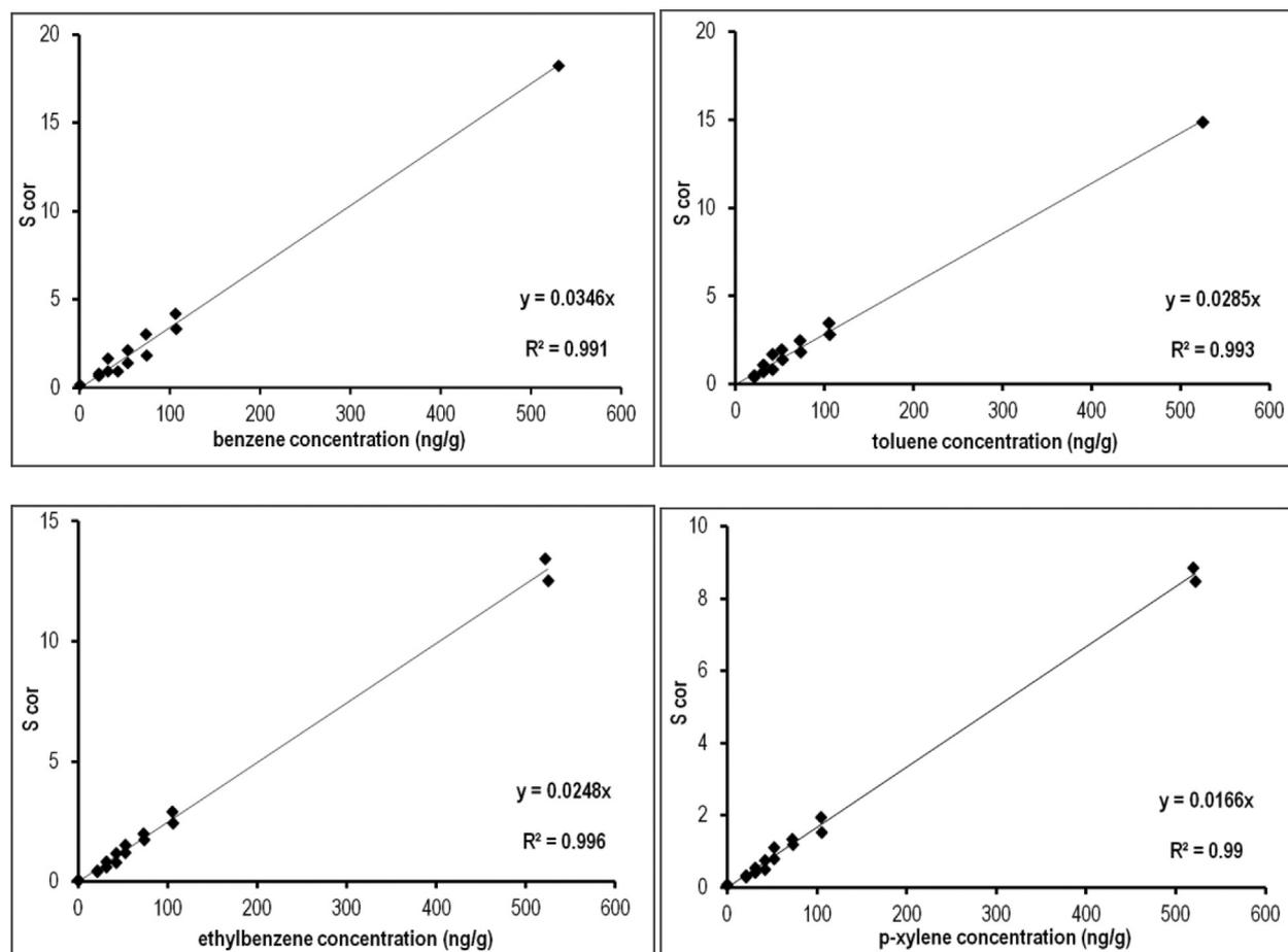
Fig. 2. Calibration curves of four hydrocarbons (benzene, toluene, ethylbenzene and -xylene). The  $S_{cor}$  (corrected area) dependence on  $c$  (hydrocarbon content per gram of capped brood or bee bread).  $S_{cor}$  was calculated as the quotient of the peak area characteristic of a given hydrocarbon and the peak area of the internal standard (n-butylbenzene).
