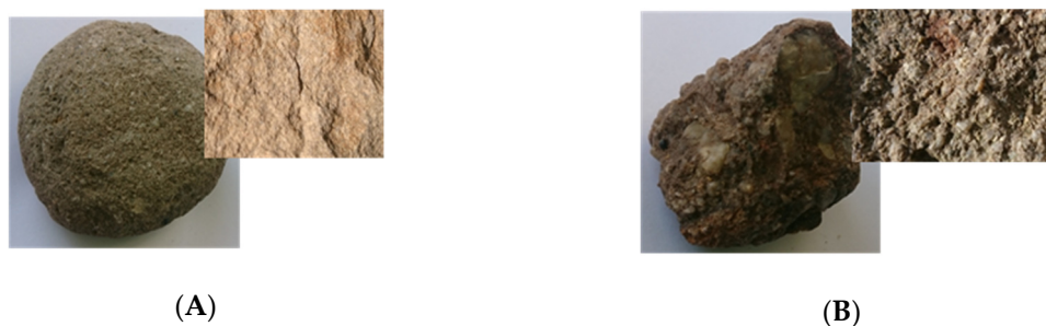
Figure 2. Gravels consisting of (A) fine-grained sandstone and (B) coarse-grained sandstone
