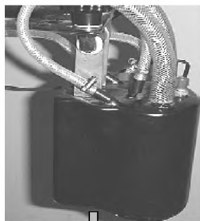
Fig. 1. Appearance of stimulating coil (core coil with water cooling) and its location over the cage for rat immobilization during rTMS stimulation (real size proportion).
