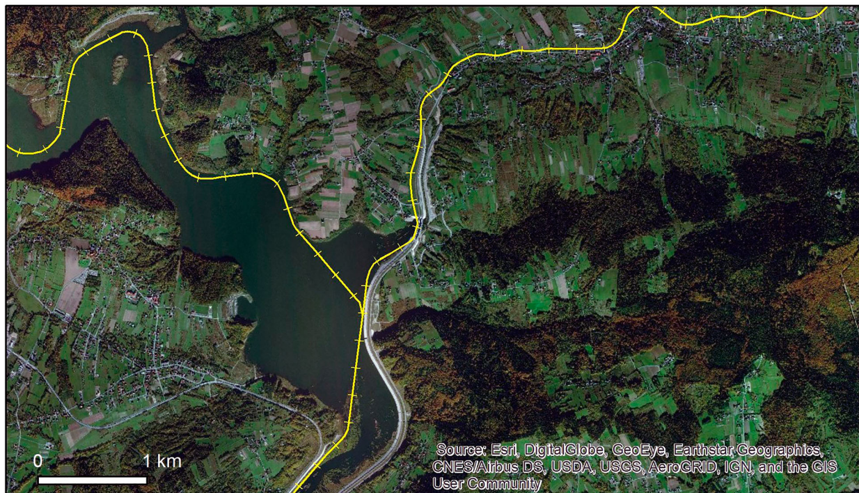
Figure 3. Reconstruction of the closed section between Wadowice and Skawce and the redesigned section between Kraków and Zakopane that was built due to water reservoir construction in the Polish Carpathians. In the database, in each case, the original shape from times of construction of the lines in 1884 and 1899 was reconstructed; source: Bing Imagery, ArcMap basemap.
