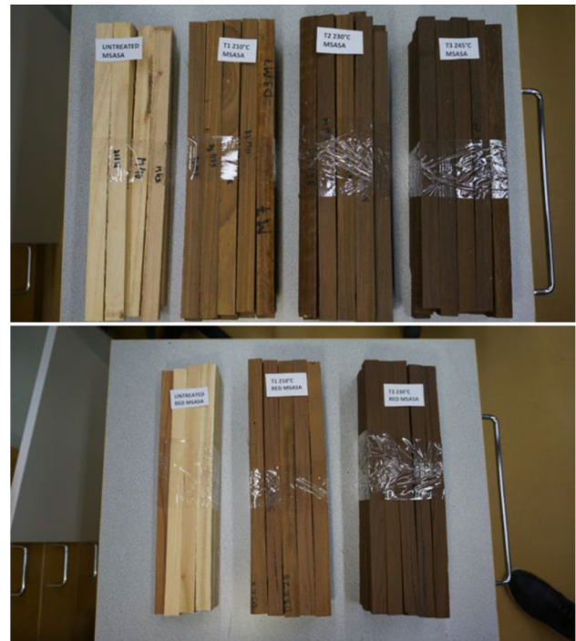
Fig. 1 Bending test specimens of B. spiciformis (above) and J. globiflora (below) showing the gradual change of colour, from left: untreated, T1, T2, and T3
